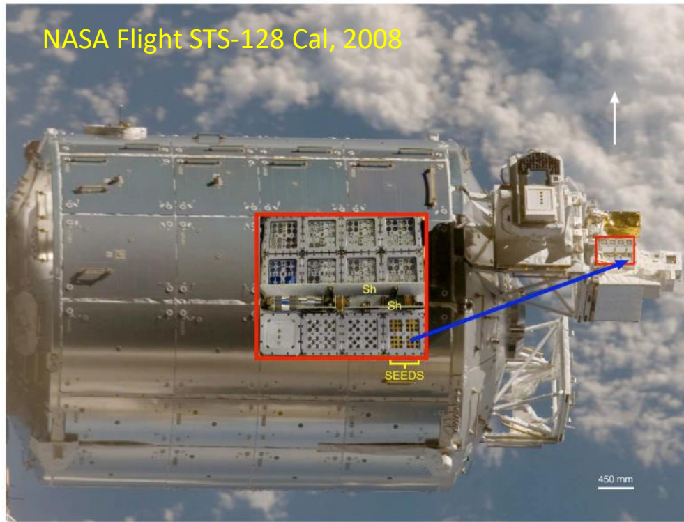
Fig. 1. EXPOSE and SEEDS on the Columbus module of the ISS (Photo courtesy NASA). EXPOSE (small red box) is on the EuTEF platform. SEEDS is covered by a protective shutter (closed in this photo, taken prior to
