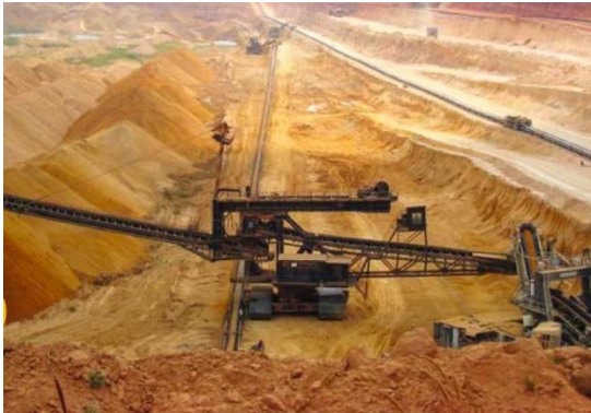
Opencast mining of phosphate rock in Togo. Most of the world's phosphate rock is extracted from open pits, as shown here, or from largescale mines equipped with drag lines or shovel/excavator systems. Credit: Alexander Ruzhichevsky
